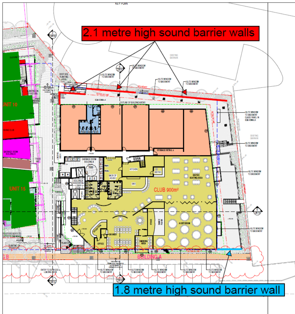
Figure 15: Location of sound barrier walls
