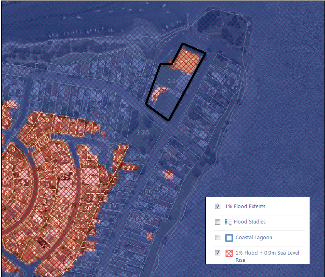
Figure 23: Flooding Impact (site shown highlighted in black).
